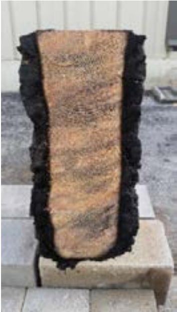
Charred CLT section. Source: Timber Frame Engineering Council
