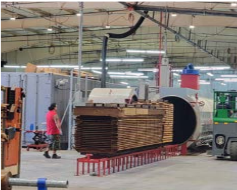
Top: CWH boards after planing and thermal treatment. Defective boards will be turned into decking. Bottom: CWH after a round of thermal treatment. Small wood slats provide airflow between boards while iron plates help to keep the wood in the place.
