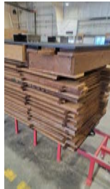
Top: CWH boards after planing and thermal treatment. Defective boards will be turned into decking. Bottom: CWH after a round of thermal treatment. Small wood slats provide airflow between boards while iron plates help to keep the wood in the place.
