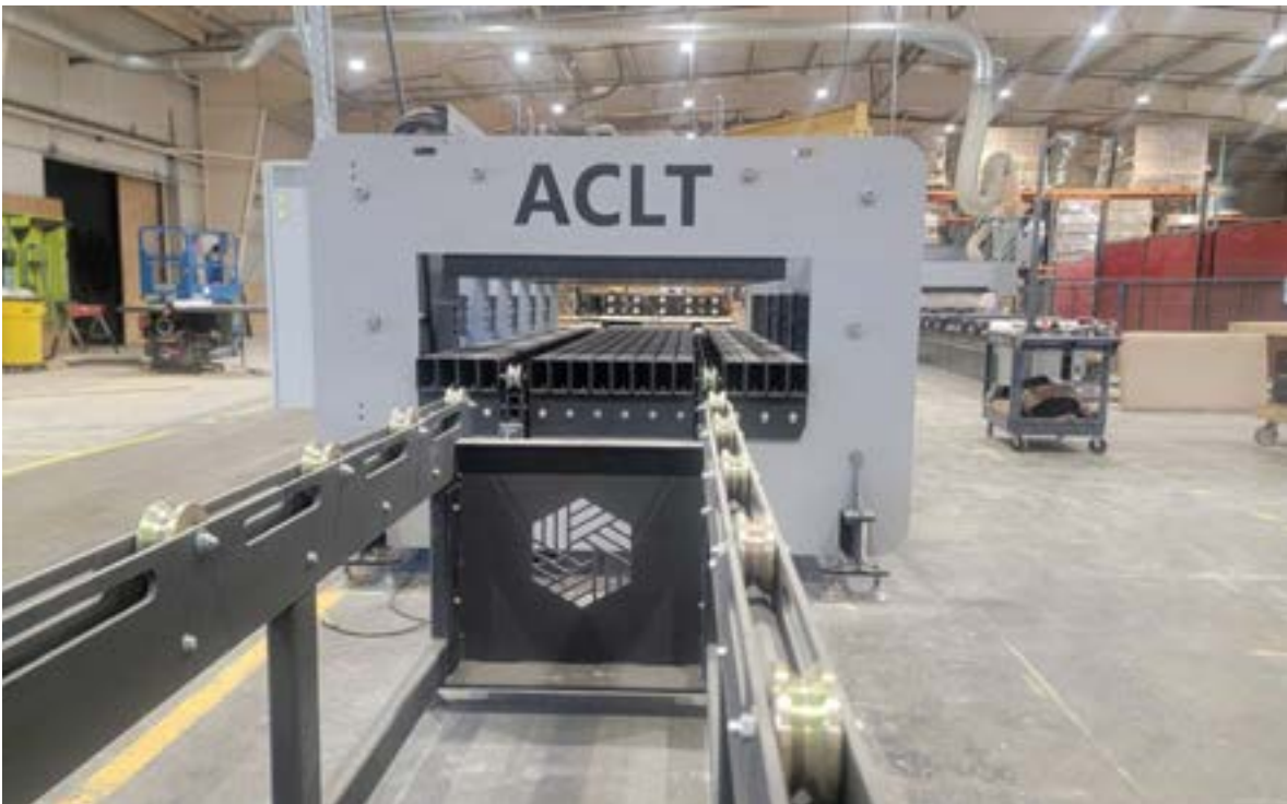
Top: Freshly laminated panels. The evenness of the press can be evaluated by the distribution of the glue seepage. Bottom: The CRTC's custom ACLT press, designed and fabricated in house. The press is designed to be significantly stronger, wider, and more even than other available commercial presses.
