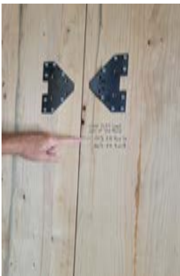
Top: Labeled two-foot panels used to construct the roof. Bottom Left: Marker lines showing panel movement under earthquake testing. Bottom Center and Right: Connections between panels.
