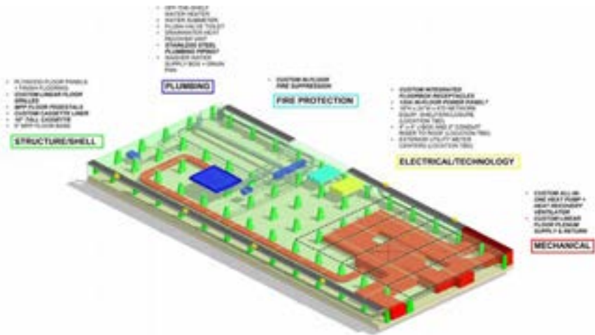
The cassette floor system, which uses mass plywood to encapsulate equipment.
